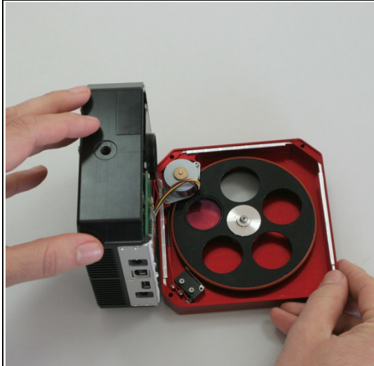
Turn down the wheel module onto the table.
