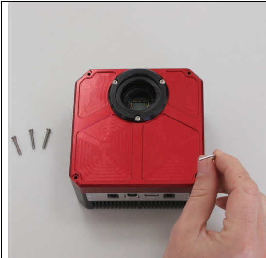
On a clean table, unscrew the 4 front screws.
