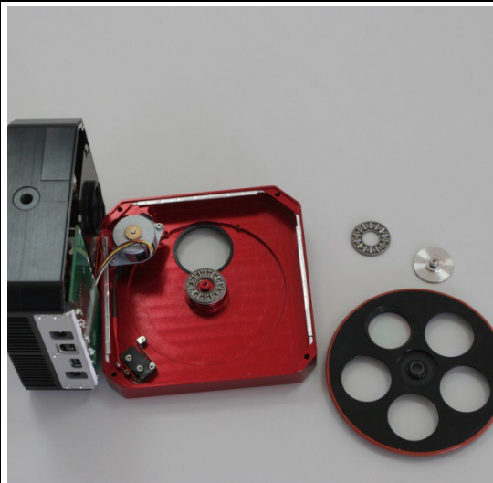
Remove the bearing by turning disk upside down. Parts should look as above.
