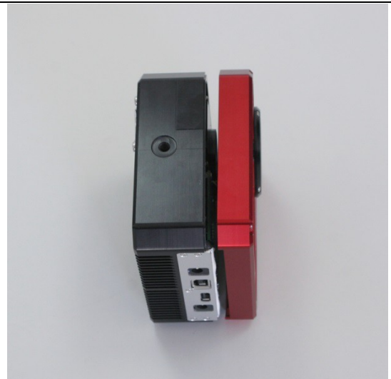
Place the camera sideways and gently separate the wheel module.
