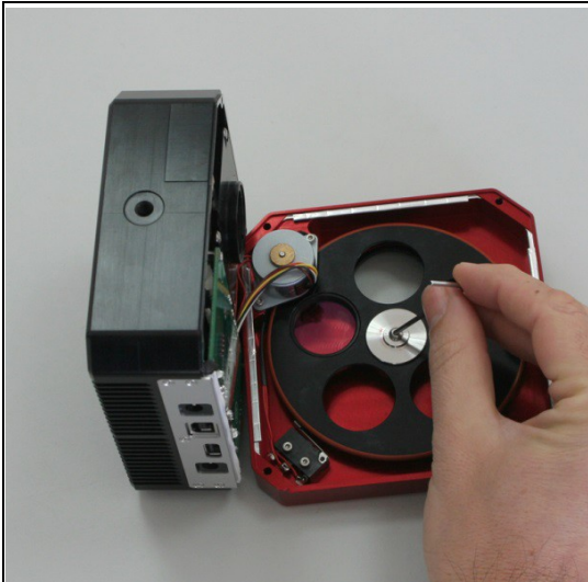
Unscrew the central holding screw.
