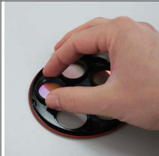
Install filters on disk
